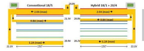
At a full 150ft. the voltage drop difference between conventional any hybrid cables is hardly noticeable. Using hybrid thermostat cable, the thermostat and the relays continue to function while using a fraction of the copper.
